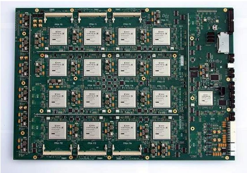
Figure 3: FPGA-based prototyping platform (courtesy of Dini Group)
