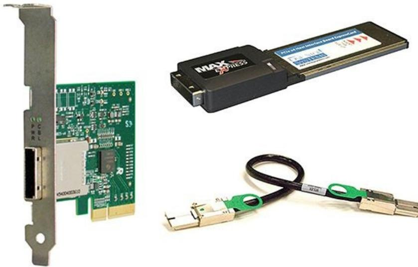
Figure 2: PCI Express cable and Express Card adapters (source: One Stop Systems)
