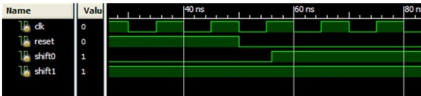
Figure 3: shift0 and shift1 are stuck at logic '1'
