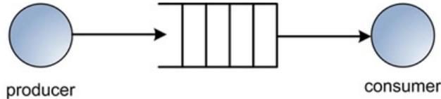
Figure 3: FIFO producer-consumer model
