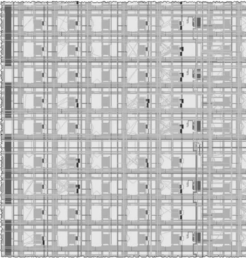
**Figure 2: FPGA routing structure**
