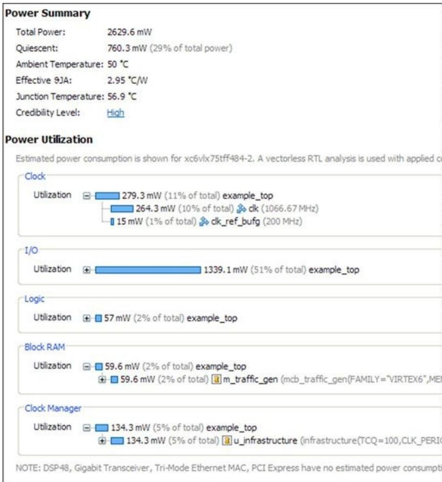
Figure 1: PlanAhead Power Estimator results
